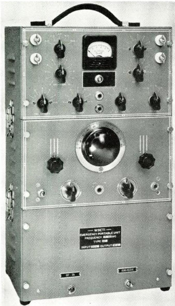
The units come apart, and yet the whole can be transported as one complete radio station.
